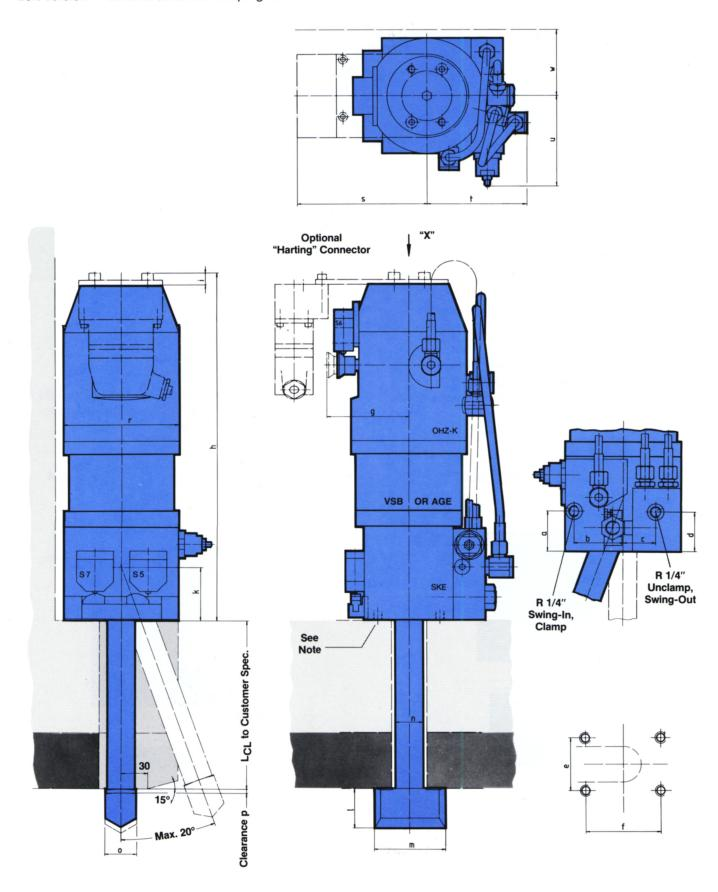
$\label{eq:Right Version} \textbf{--} \textbf{All limit switches and plug connectors are on the right}.$
