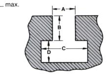
**Note:** Please give depth of throat dimension "T" even if using a standard T-slot.
