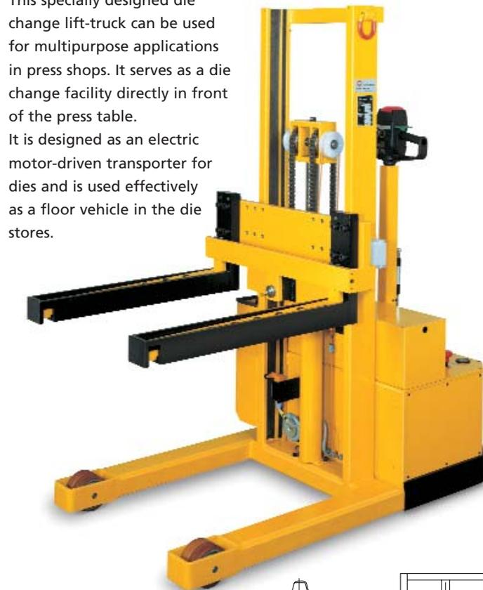
By lowering in a coupling, the front of the carrying forks is docked with the press bed for the purpose of transferring dies in loading and unloading operations.
